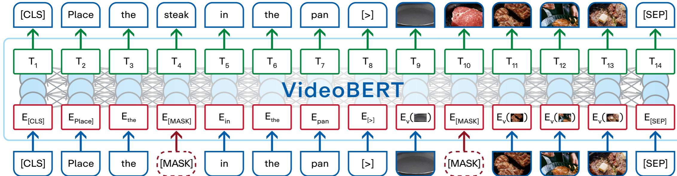
The AI model “VideoBert” simultaneously analyses images and text in videos. The system is trained by omitting parts from the audio channel—such as “steak”—which VideoBert then has to guess. The same happens in the image channel (see illustration). After training, the model can predict both forthcoming actions and speech in the video.
