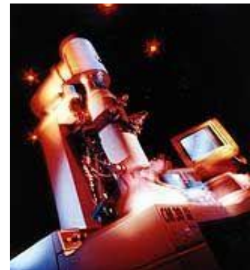
The special electron microscope for atomic electron holography. Built to the specifications of the Tübingen-based scientists at Philips, it currently allows the holographic depiction of structures with a fineness of 0.13 nm. The target is 0.1 nm. (Photo: Peter Allert)
